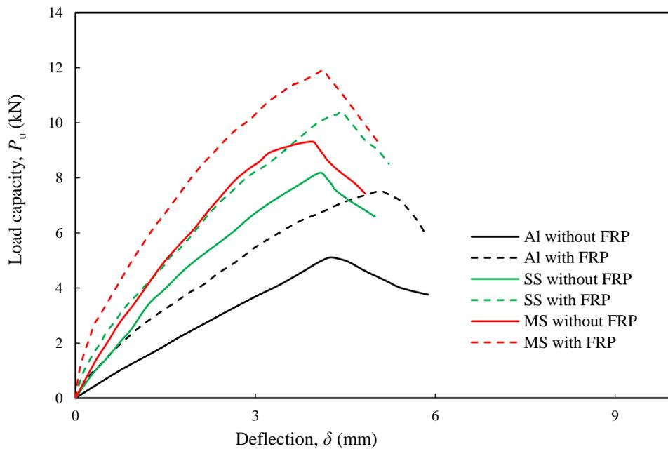
Fig. 8: Comparison of ultimate capacity for reference and strengthened section
