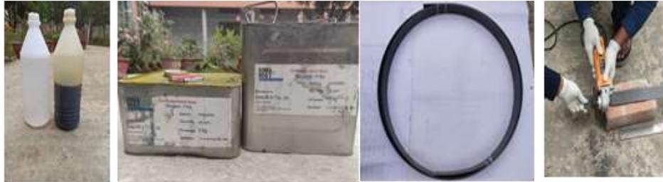
Fig. 1: Primer, Saturant, adhesive and CFRP Fabric
