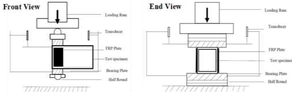
Fig. 5: Schematic view of ETF loading test arrangement
