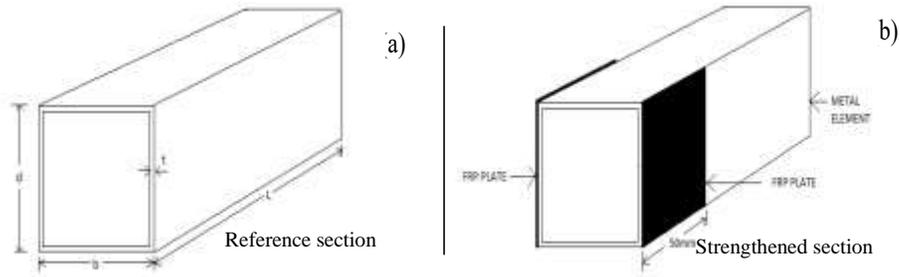
Fig. 2: Dimension of tubular metal section and FRP strengthen specimen for ETF loading
