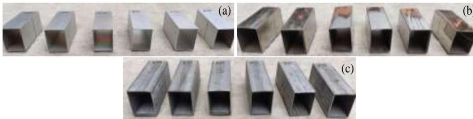
Fig. 3: (a) Aluminium, (b) Stainless steel, and (c) Mild steel specimen for ETF test specimens
