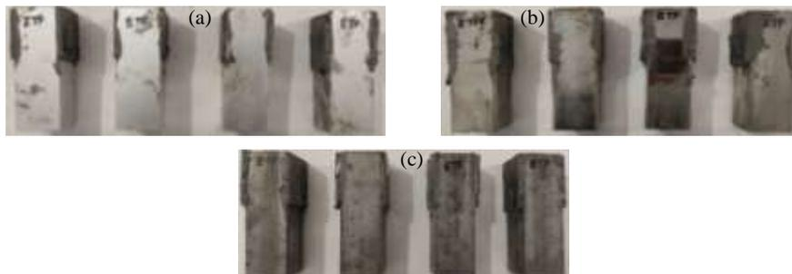
Fig. 4: CFRP plate strengthened (a) Aluminium, (b) Stainless steel and (c) Mild steel specimen for ETF test specimens
