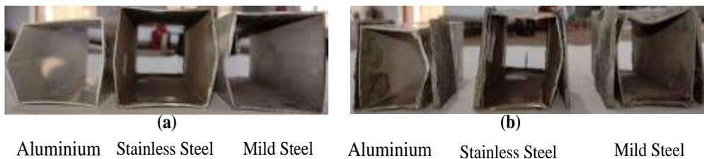
Fig. 7: Specimen after failure (a) reference sections (b) FRP strengthened sections
